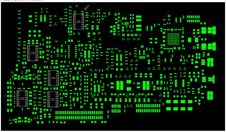
You can see the problem where the arrow is pointing. A component with a larger number of pads was detected incorrectly.
